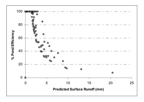
Figure 3: The predicted variation in sediment pond efficiency with event size.
